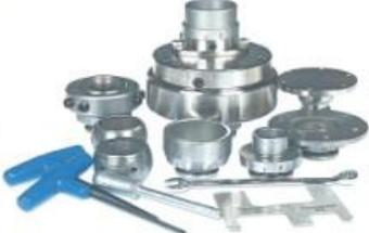
The main feature of the chuck is its infinitely variable axis setting capacity. With an offset range of 0 to 30mm, each setting gives a different turning axis. In addition to this the rotating cup chuck allows you to create an even wider variety of shapes, depending on the chosen axis. The optional ball chuck allows the work piece to be swivelled up to 15° off axis for even more flexible turning.
